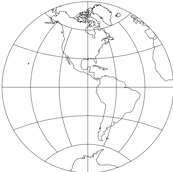
Figure 61: Nicolosi Globular projection, with shorelines and 30° graticule. Central Meridian 90° W (+proj=nicol +lon_0=90w).
