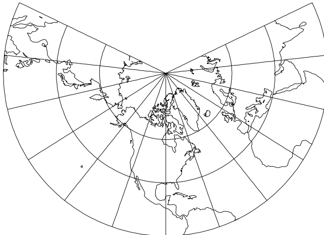
Figure 39: Perspective Conic projection, with shorelines and 30^\circ graticule. Central Meridian 90^\circ W. and standard parallels at 20^\circ N and 60^\circ N (+proj=pconic +lon_0=90w +lat_1=20n +lat_2=60n).
