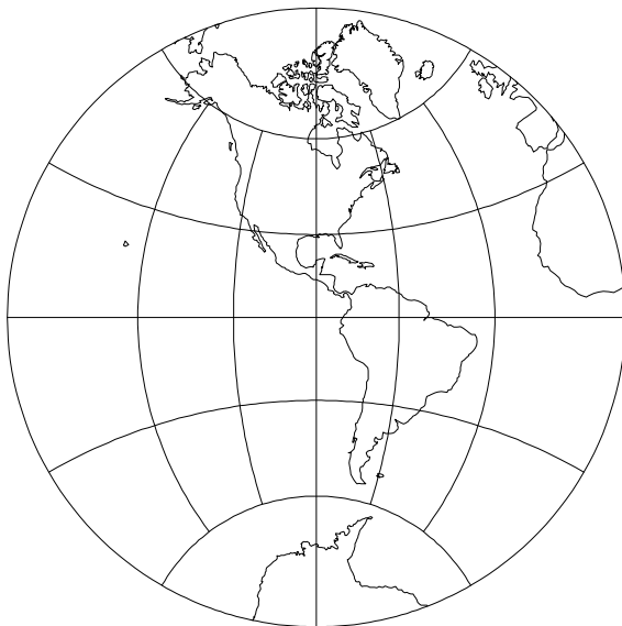
Figure 71: Lagrange projection, with shorelines and 30° graticule. Central Meridian 90° W. ( +proj=lagrng +lon_0=90w +W=1 )
