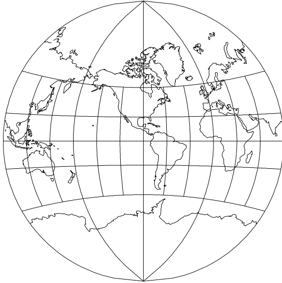
Figure 66: Van der Grinten I projection, with shorelines and 30° graticule. Central Meridian 90° W (+proj=vandg +lon_0=90w).
