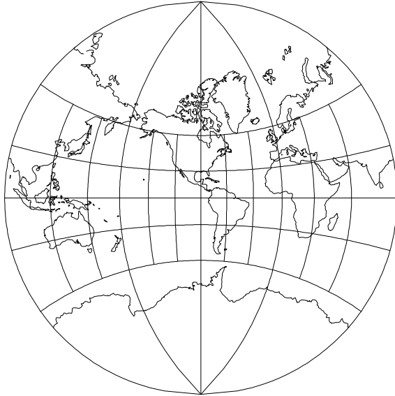
Figure 70: Lagrange projection, with shorelines and 30° graticule. Central Meridian 90° W. ( +proj=lagrng +lon_0=90w )
